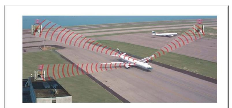
Transponder signal reception from more than 3 ground sensors Aircraft position identification by using TDOA (different time of arrivals) Mode A/C and Mode S availability
